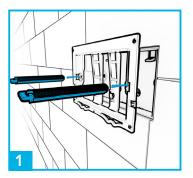
Attach the button bracket using the clips provided
