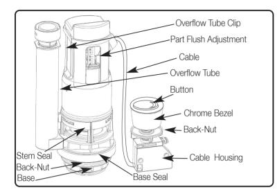
To adjust the full flush volume, raise/lower the full flush adjustment as shown; the lower the slide is set, the higher the flush volume will be.
